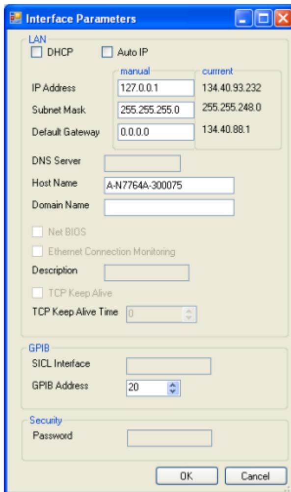
**Figure 36** Interface Parameters
